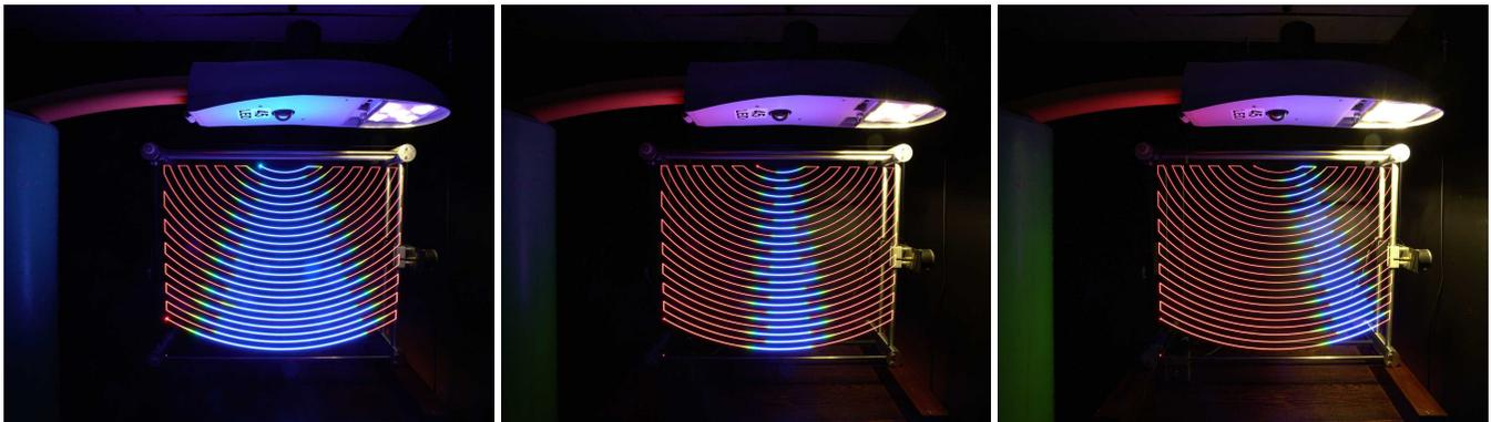
Figure 1: Metaveillography of smart street light with built in camera, wide, then zoomed in, then panned to the right.
