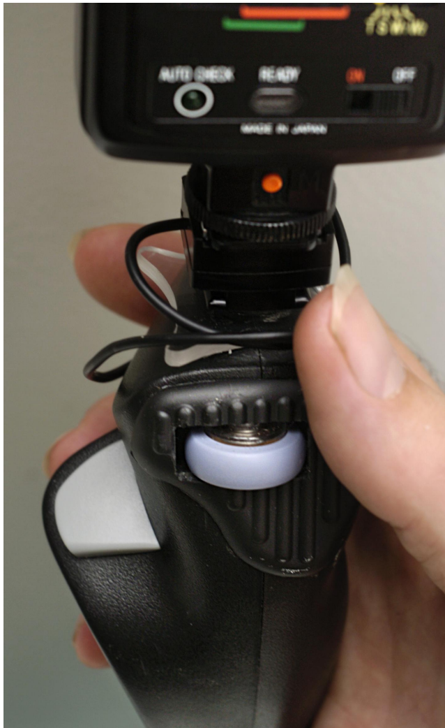
Fig. 4: The “white balance” thumb wheel on the terrometer.
