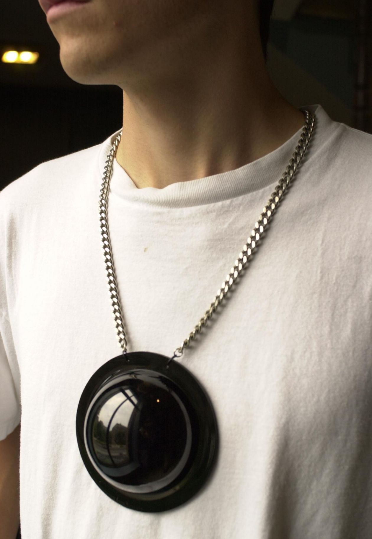
Wearable camera with fisheye lens, various sensors, and wireless communications Copyright (C), Steve Mann, 1998
