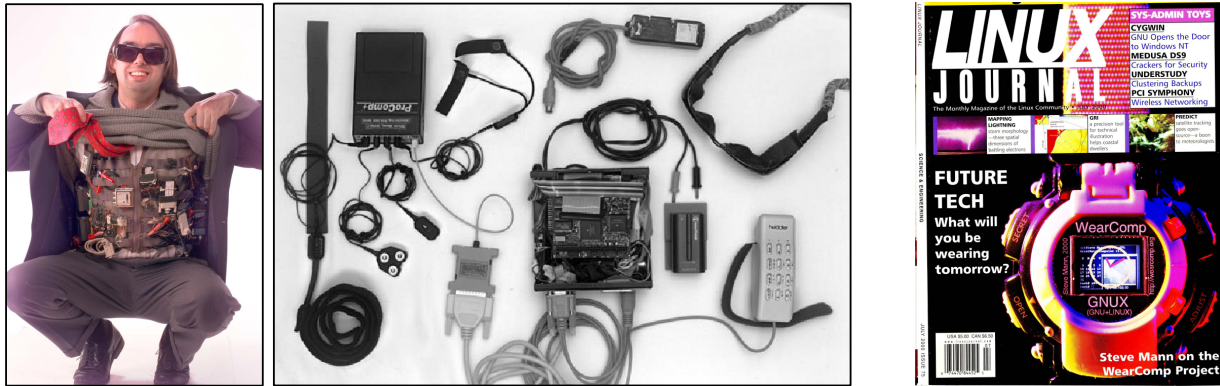
Figure 4: My Quantimetric Self-Sensing (QSS) system. Left: A 1996 sensing vest and eyewear measured and processed respiration, ECG (electrocardiogram), EEG (electroencephalogram), EMG (electromyogram), GSR (galvanic skin response), audio and video of the surroundings, and many other signals. This system was presented to Kevin Kelly at the WiReD offices in San Francisco, where he called it “Quantified Self.” Right: miniaturization of the apparatus resulted in the world’s first smartwatch in 1998, featured in Linux Journal , July 2000.
