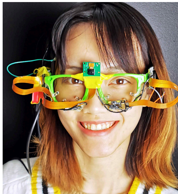
Fig. 1: The wearable glass design for prosopagnosia worn by a subject.
