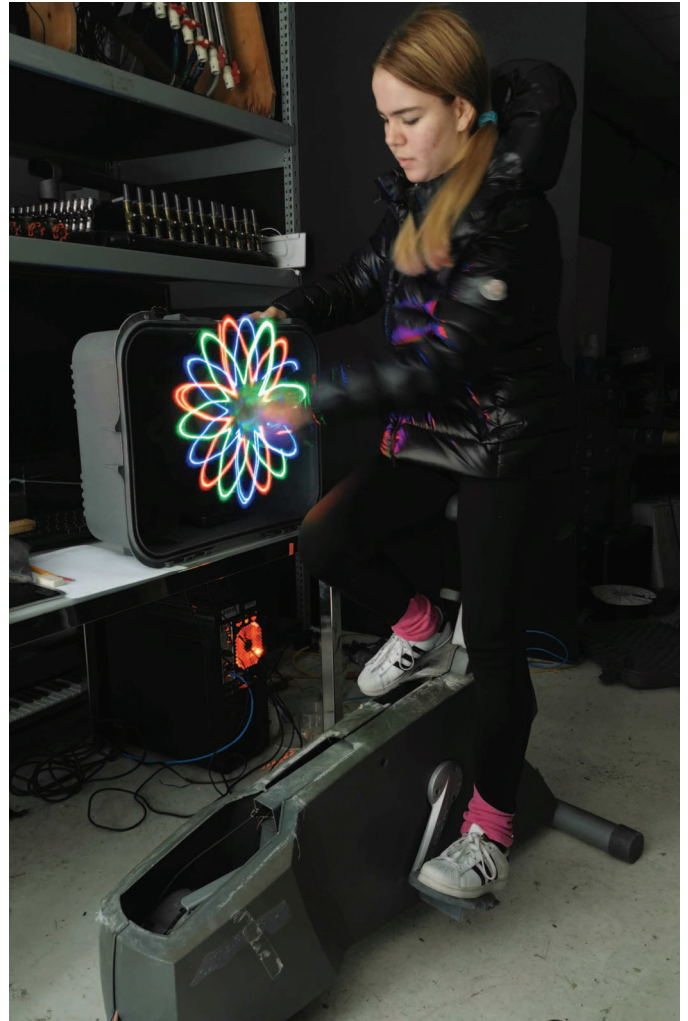
Fig. 10. Exploring the interconnection between electric machines. Here are two Lundell machines, one in a stationary bicycle and the other hand-cranked. The hand-cranked machine features a rotary SWIM (Sequential Wave Imprinting Machine).
