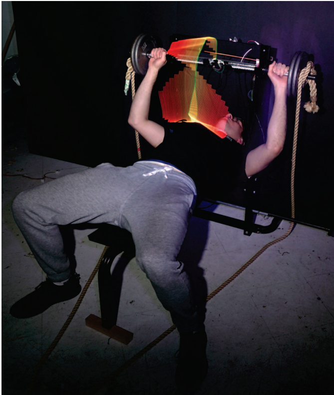
Fig. 2. A user of our integral kinesiology system performing a bench press. A SWIM [19] (Sequential Wave Imprinting Machine) is used to guide the user through the exercise by way of real-time visual feedback on form. Note the rope which provides dissipative friction (energy loss) to dampen the inertia of the weights. It is also connected to a spring, so that all 3 forms of impedance are present.
