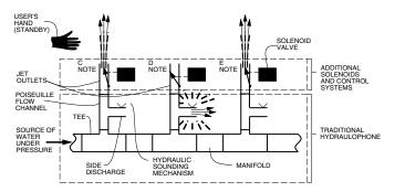
Fig. 2: Solenoid valves added to a traditional hydraulophone to make it into a player-hydraulophone: The hydraulophone works like a "player-piano" and plays a portion of a song. Here it is shown playing one note (D). It does this by closing the valve associated with the D note, which diverts water to the hydraulic sounding mechanism. To the user, it appears as if a hidden player is blocking that one jet to make it sound.
