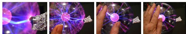
Figure 6: Plasmaphone : Sound is produced by plasma. A number of different kinds of plasmaphones have been built by the author, with various kinds of pickups. The one shown here uses optical pickups (wrapped in foil for shielding from high voltage interference) on each of several plasma balls. As more fingers come closer to one of the plasma balls, plasma is drawn away from a pickup, resulting in dramatic changes in the sound produced.
