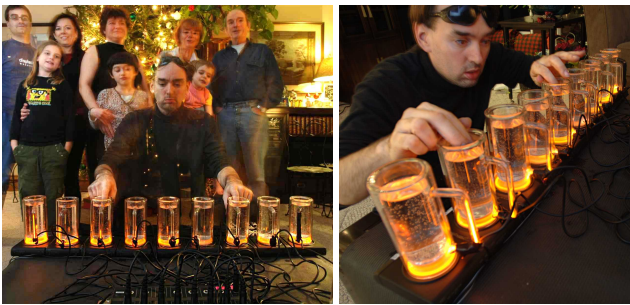
Figure 7: Another variation of the plasmaphone at the 2006 PineHill Christmas Concert, December 25th: Commercially made high voltage plasma mugs bought from a novelty store are designed to be filled with water and touched. The author bought nine of these “plasmugs” and made them into a highly expressive “plasmacoustic” instrument.
