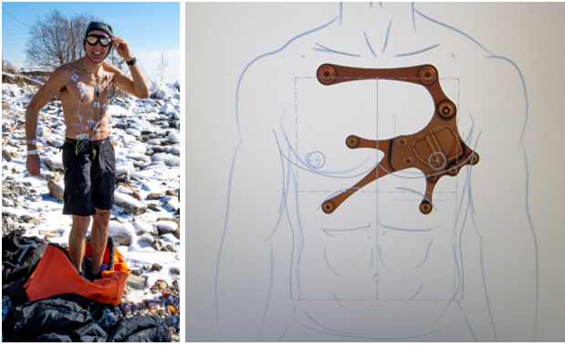
Figure 36. World's most advanced underwater heart monitor and augmented reality biofeedback system for swimmers (Left) prototype (thanks to Dan Bowman for picture). (Right) Design of the world's most advanced heart monitor with full 12-lead ECG plus realtime wearable ultrasound, and a camera that can "see" into the water while swimming. The vision system uses AI and machine learning to anticipate activities and estimate expected heart activity based on surroundings, and automatically flag any anomalous cardiac activity.
