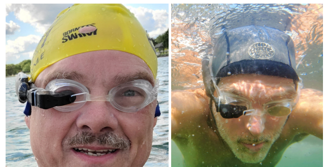
Figure 23. Vuzix Smart Swim underwater augmented reality system capable of displaying maps, wayfinding, etc., as well as live video feed from overhead drone for the SafeSwim [43] project.
