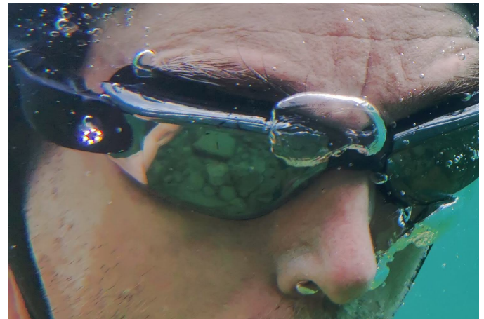
Figure 22. Custom-made underwater augmented reality eyeglass with wearable camera, underwater brain-sensor (Blueberry X Technologies brain sensing pod), and augmented reality display [42].
