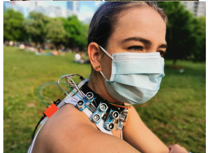
Figure 8. Social-Distancer™ art installation at DECONism Gallery for DECONference 2020 in collaboration with the Marshall McLuhan Centre for Culture and Technology. A more practical version was built as a necklace from 12 sonar devices arranged in a clock-like pattern to warn the wearer of the direction of approach of social-distance violators [13].
