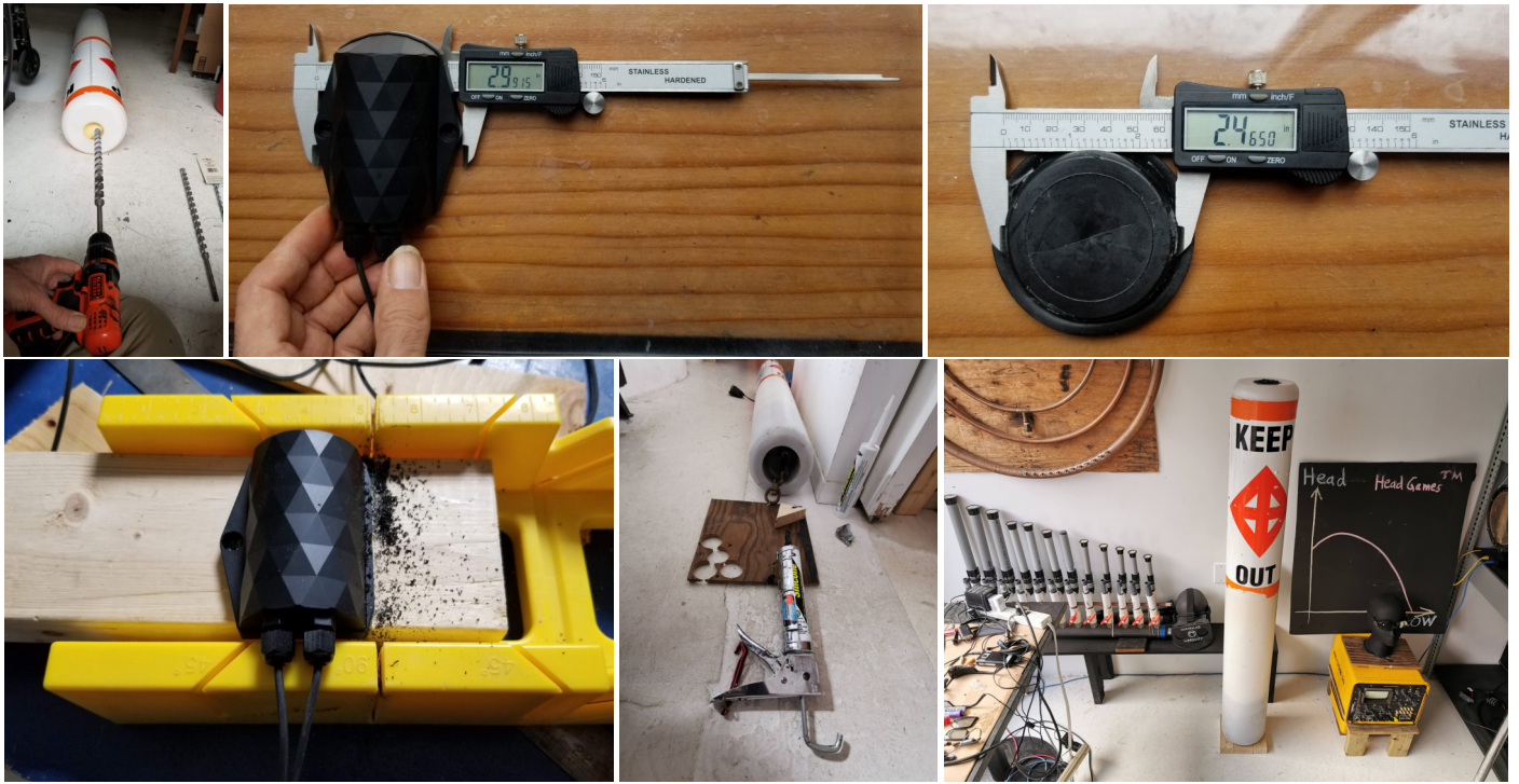
Figure 14. Building the Smart Buoy prototype. We first drilled out an existing buoy and then used cord seals having the computer and radio and antenna unit inside the hollow of the buoy and the sensor hanging down into the water. One lesson learned is that most buoys have only a very small opening, yet most sensing equipment is quite large. Here the sensor was almost 3 inches at its fattest point and would not fit through a standard 2.465 inch opening, so we had to trim it down while maintaining its waterproofness. (Bottom right) pictured at our lab with some of the other artefacts of our research: hydraulophone, underwater oscilloscope, and chalkboard illustrating HeadGames™. (system for teaching hydraulic head as a function of flow.)
