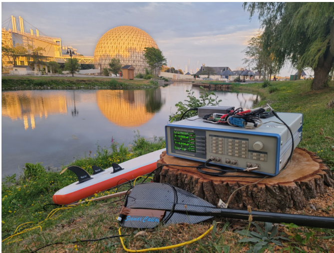
Figure 33. Experimental setup with lock-in amplifier, hydrophones, and SUP (Stand-Up Paddleboard).
