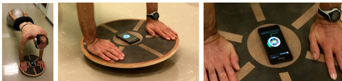
Fig. 10. Example with multidimensional Integral Kinematics in the form of pushups on wobble board which must not touch the floor along any of its perimeter (sensed, along with time-integrated tilt), while feet are balanced on a fitness ball.
