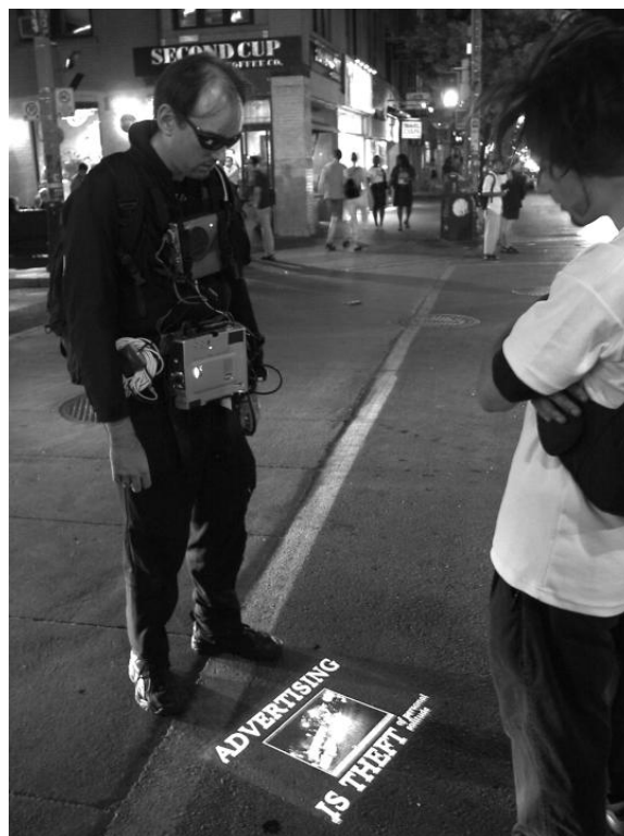
Figure 1: The wearable apparatus contains a 1 GHz P3 CPU, rendering engine, high-power mercury vapour arc lamp data projector, within a black flame-retardant Nomex (TM) uniform custom tailored to fit the wearer. Here a person can see his own image together with other computer generated material.
