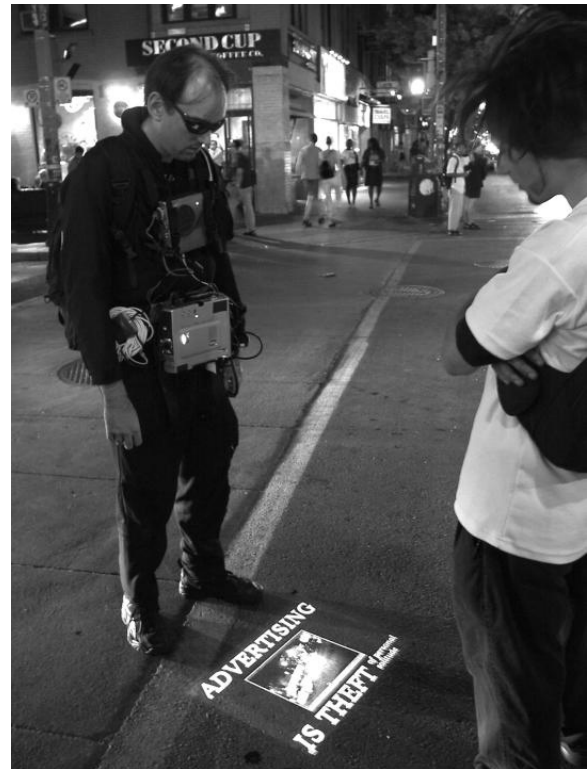
Figure 1: The wearable apparatus contains a 1 GHz P3 CPU, rendering engine, high-power mercury vapour arc lamp data projector, within a black flame-retardant Nomex (TM) uniform custom tailored to fit the wearer. Here a person can see his own image together with other computer generated material.
