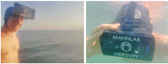
Fig. 6: The MannLab Mersivity VR/AR/XR headset, pictured here at one of the three beaches under test, was used for realtime visualization of spatially-varying beach water characteristics, “heatmap” overlays, etc., while swimming in the water.
