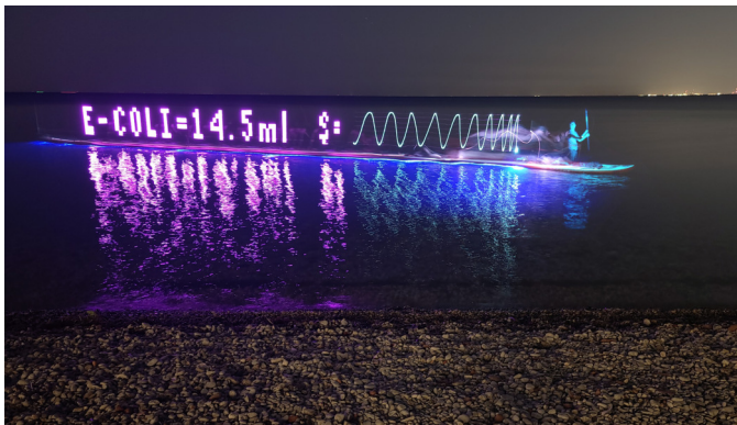
Fig. 8: Demonstration of SWIM stick on SUP where text indicates the E-Coli levels of the beach, obtained from the official city of Toronto website. Following the text, a fixed-frequency sine wave indicated the speed of the SUP. As can be seen in the photo, the SUP moves slower as it travels from left to right, as shown with an apparent increase in frequency in the long exposure photo.
