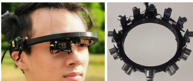
Fig. 4: Left image: Vironment reading blood pressure, pulse, respiration rate, and temperature. Right image: Social-distancing sonar necklace prototype which is an optional accessory for the Social Distancer function of Vironment.
