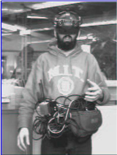
Figure 6. My early 1990s apparatus for wearable, tetherless, computer-mediated reality included a color stereo head-mounted display with two cameras. The intercamera distance and field of view approximately matched my interocular distance and field of view with the apparatus removed. Communications equipment was worn around the waist. Antennas, transmitter, and so forth, were at the back of the head-mount to balance the weight of the cameras in front.
