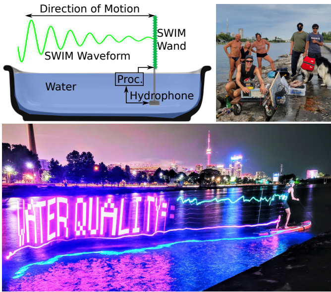
Fig. 1: Schematic diagram of the linear SWIM, an early form of WaterHCI (Water-Human-Computer Interaction) invented in 1974, together with more recent photographs showing its use upon a vessel (SUP = Stand-Up Paddleboard) for applications in water safety. Top right: photograph of the SUP-shore communications and realtime processor. Bottom: photograph of the time-varying waveform in green, with axis-labeling (“WATER QUALITY”) in magenta, as light trails left by the paddleboard and paddler visible at the right side of the photo. By sensing water quality in real time, important aspects of aquatic safety can be sensed and communicated immediately.
