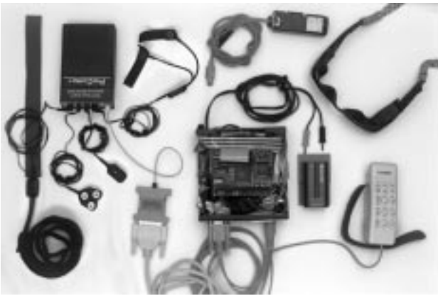
Fig. 7. Author's personal imaging system equipped with sensors for measuring biological signals. The sunglasses in the upper right are equipped with built-in video cameras and display system. These look like ordinary sunglasses when worn (wires are concealed inside the eyeglass holder). At the left side of the picture is an eight-channel analog-to-digital converter together with a collection of biological sensors, both manufactured by Thought Technologies Limited, Canada. At the lower right is an input device called the "twiddler," manufactured by HandyKey, and to the left of that is a Sony Lithium Ion camcorder battery with custom-made battery holder. In the lower central area of the image is the computer, equipped with special-purpose video processing/video capture hardware (visible as the top stack on this stack of PC104 boards). This computer, although somewhat bulky, may be concealed in the small of the back underneath an ordinary sweater. To the left of the computer is a serial-to-fiber-optic converter that provides communications to the eight-channel analog-to-digital converter over a fiber-optic link. Its purpose is primarily one of safety, to isolate high voltages used in the computer and peripherals (e.g., the 500 volts or so present in the sunglasses) from the biological sensors which are in close proximity, typically with very good connection, to the body of the wearer.
