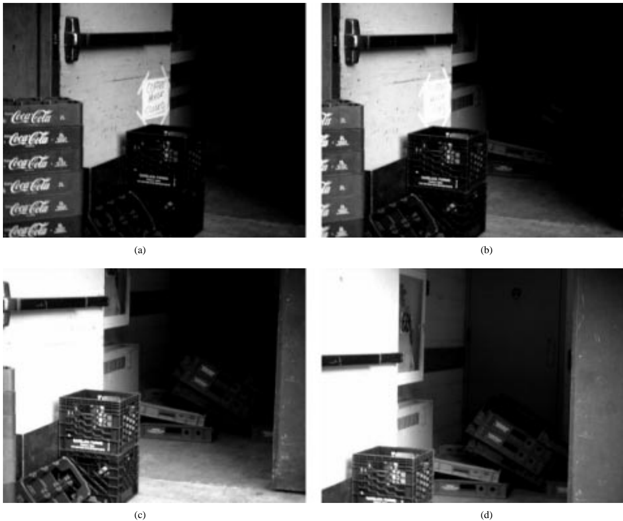
Fig. 8. The “fire-exit” sequence captured using a covert eyeglass-based personal imaging system with AGC. Here, every third frame of the ten-frame image sequence is shown. As the camera pans across to take in more of the open doorway, the image brightens up showing more of the interior, while, at the same time, clipping highlight detail. (a) Frame 0 shows the writing on the white paper taped to the door very clearly, but the interior is completely black. (b) In Frame 3 the paper is obliterated—it is so “washed out” that we can no longer read what is written on it. Although the interior is getting brighter at this point, it is still not discernible in Frame 3—we can see neither what is written on the paper, nor what is at the end of the dark corridor. However, as the author turns his head to the right, pointing the camera into the dark corridor, more and more detail of the interior becomes visible as we proceed through the sequence, revealing the inner depths of the long dark corridor, and showing that the fire exit is blocked by the clutter inside.
