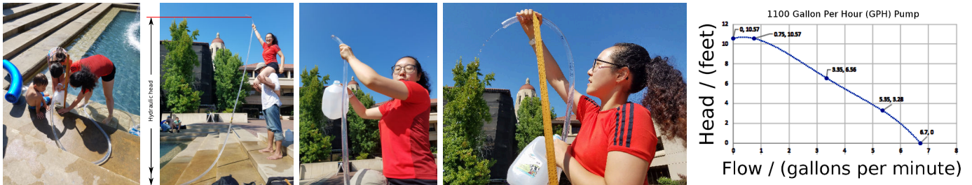
Fig. 3. Head Games: measuring flow rate as a function of hydraulic head, to plot the characteristic curve of a water jet. Materials required: water pump, long hose (preferably transparent so students can see the water in it), ruler or tape measure, and measuring cup/jug (i.e. measuring “gallon”). Using a long hose, for each height of the far end of the hose, the time to fill a one-gallon jug is measured. From this measurement is calculated the flow rate (gallons per minute). This may be done by either inserting a small low-voltage submersible pump into the fountain, to supply the hose (here an 1100 GPH Rule ITT pump), or by holding by hand against one of the water jets, as shown in Fig. 6, or by insertion into a water jet by careful choice of hose diameter, as shown in Fig. 7. It is interesting to note, that for many systems, the deadhead is less than the maximum head (i.e. the curve increases and then decreases again.). The deadhead point is the point at which the hose is held so high that no water comes out of it (i.e. the pump is pushing up to the maximum water column it can sustain, as shown in Fig. 5). Often there are two points where this happens, with an even higher amount of head in between them. The “teach beach” concept makes this teaching fun and playful in the context of Stanford University’s “fountain hopping” tradition. Pictured here are Prof. Mann’s students Cindy and Adnan (who is also the founder of CG Blockchain and Blockchain Terminal, http://bct.io ).
