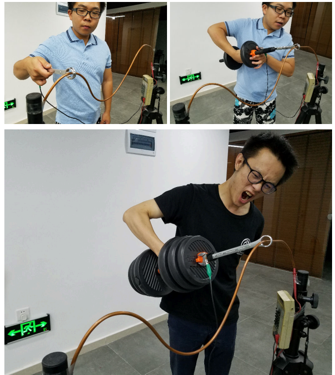
Fig. 1. Left: Undigital buzzwire game. A serpentine length of wire (copper refrigeration tubing) is connected to one terminal of a capacitance meter (proximity sensor), and the other terminal is connected to an open-ended wrench. Distance between the wrench and the wire is sensed, and the distance from the center of the wrench is calculated. This calculated center-distance is then integrated to obtain absement. Score is based on the reciprocal of the absement. This game tests dexterity. Right: By adding weights, we turn this game into a physical fitness activity that measures and develops “dextrength”, i.e. a combined simultaneous exertion of dexterity and strength. The MannFit™ system [5] is a commercialization of this technology in which absement is integral to building combined simultaneous strength and fine-motor control. Bottom: Extreme strength combined with fine-motor control, by adding massive quantities of weight.
