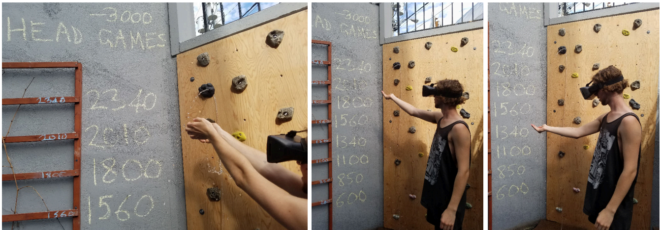
Fig. 8. Head Games™ climbing wall. Here a participant experiences head by touching the water jet from various heights. Calculations are rendered in the virtual world, where the eyeglass actually operates in a “multimediated reality” mode, using video see-through and overlay of water jet attributes with actual water. Left: deadheading the jet results in much higher head, but coming away from it results in much less head. Middle: the head increases again as we move down. Right: further down the head increases, due to further potential energy transferred to kinetic energy.
