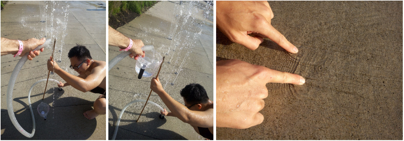
Fig. 6. Head Games played by connecting a hose to one of the water jets in a splash pad aquatic play area. A ruler is used to measure the hydraulic head (height of water column) and a measuring cup is used to measure the amount of water flowing in a given time to determine flow rate. In our final teach beach™, we envision that the jets would be designed for easy coupling to hoses which would be lent to participants so they don't have to bring their own as we did here. Rightmost: exploring interference patterns between waves formed by Karman vortex shedding in bluff bodies (in this case, fingers) inserted into moving water. Karman vortex shedding is the principle of operation of some hydraulophones. The fingers are roughly cylindrical, and the Strouhal number ( St ) (dimensionless quantity characterizing oscillating flow mechanisms) of a cylinder is approximately 0.18.
