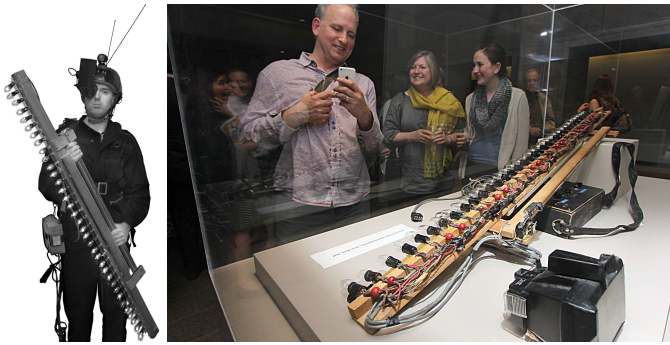
Fig. 3. Sequential Wave Imprinting Machine (SWIM) consisting of a linear array of electric light bulbs connected to a wearable computer and wearable lock-in amplifier. This functioned like a giant “paintbrush” to create an augmented reality world from the physical phenomenology of metaveillance [16], [21], “painting” with the light to expose the human eye or photographic film to the camera’s metaveillance field. Rightmost: World’s first wearable augmented reality computer (built by S. Mann in 1974) on exhibit at National Gallery in 2015.
