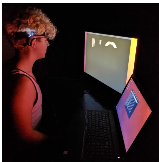
Fig. 9: The setup of the display, control computer (running Ubuntu™GNU/Linux operating system), Muse™EEG system, and participant for the "NO CAMERAS" imaging trials.
