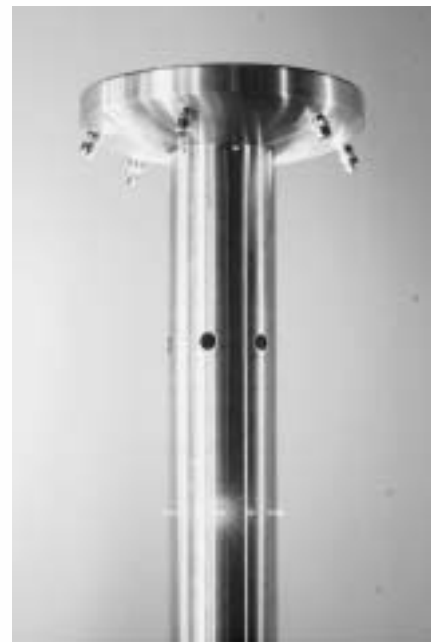
Fig. 4. Sensor-operated column shower in which five of the six nozzles are visible. (© Steve Mann) Also visible are three of the six small round viewing windows and some of the 12 laser diode body scanners, two being positioned below each viewing window.
