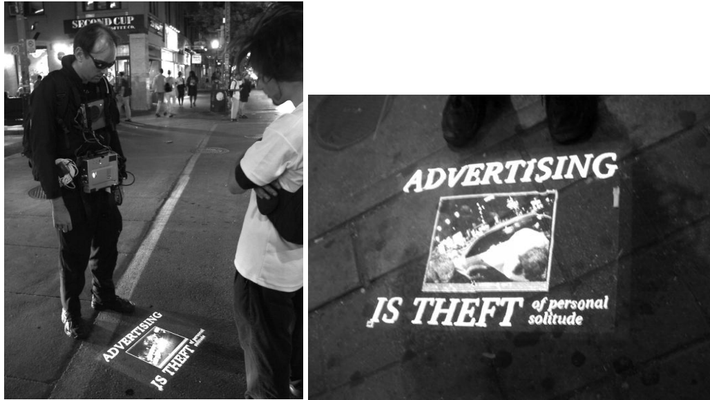
Fig. 1. (a) The wearable device contains a 1 GHz P3 CPU, rendering engine, high-power mercury vapour arc lamp data projector, within a black flame-retardant Nomex uniform custom tailored to fit the wearer. Here a person can see his own image together with other computer generated material. (b) Close-up view showing the output of the high intensity data projection system.
