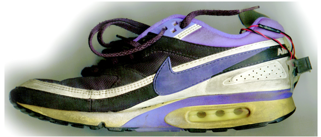
Figure 1: Power-generating shoe prototype made by author in collaboration with Nike: Piezoelectric pads running embedded in the shoe generate electricity from footsteps.
