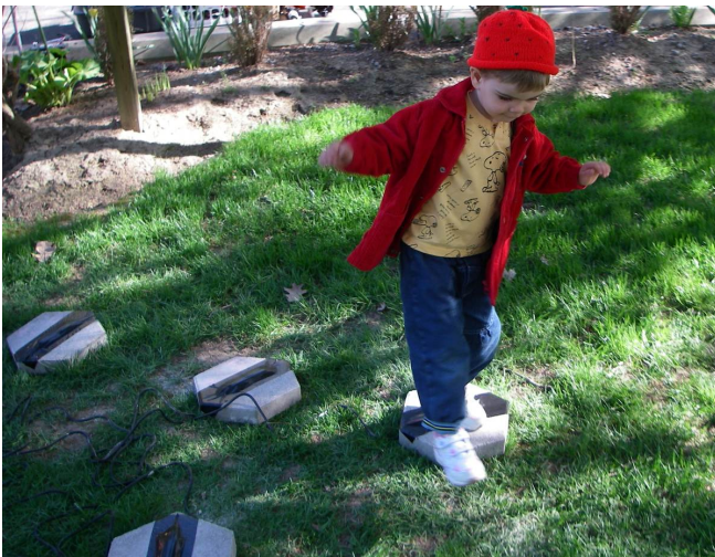
Figure 7: Garden stone slabs each define one beat in the song: As people walk on the slabs they “step out” the song by way of a computer-controlled pipe organ sculpture made from grey PVC electrical conduit pipes hanging from a tree adjacent to the garden.
