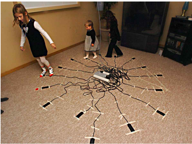
Figure 4: Experimental prototype: I first tried various arrangements of sixteen pressure sensors, taped to the floor, indoors. I designed, built, and programmed a system to sequence through one beat note of a song for each foot step.
