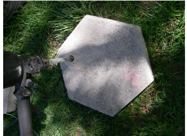
Figure 5: Preparing patio stones for being equipped with the sensors of Fig. 4: I drilled an off-center hole, and then bonded a pressure sensor in the center of the stone, with a wire passing down through the hole, to connect the sensor underground to the central processor that I mounted in a weatherproof electrical box. Using technology similar to a wearable computer (low-power battery operation) the entire sculpture can run off a small solar panel or small battery.
