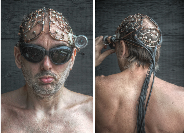
Figure 5: The MindMesh TM BCI (Brain Computer Interface) FPGA mesh-computing architecture has 64 electrodes, so that various items such as the Kinect or more conventional cameras can be “plugged into the brain”.
