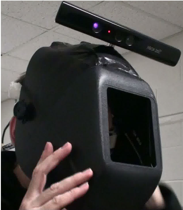
Figure 2: Our wearable configuration with a Kinect and vibrotactile actuators mounted on a welding helmet. A welding helmet was chosen because of its comfort, its electronically controllable blindfold (which defaults to transparent upon power failure), and because, other work, we are using this system in welding applications.
