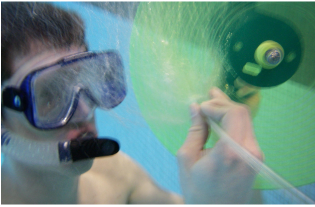
Figure 6: Underwater testing one of our hydraulic gramophone disks: After laser-cutting our record, we tested it by spraying water into the grooves. The result is a completely mechanical sound sample storage media that’s playable with a stylus consisting of a water jet (in this picture we’ve put some air into the water jet to make it visible underwater).
