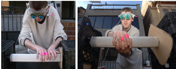
Figure 10: Polyphonic friction-idiophone as a continuously variable sampling surface for morphing stylus: A spinning aluminum cylinder with a specially textured surface produces sound picked up by a wireless contact microphone inside the cylinder.
