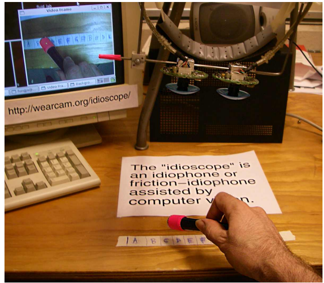
Figure 2: Making a bell-like sound from hitting a desk: A computer music system that is not an electronic instrument. Sound originates acoustically, and the role of the computer is merely for post-processing (much like a Wah Wah pedal on a guitar). The center frequency of the filter's passband varies with position, as detected by the overhead camera rig. Note the wearable stereo camera rig hanging from a fixed location. The cameras can be mounted to a tripod, or worn by the player.
