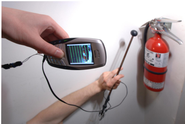
Figure 4: A 12-bar idioscope running on a camera phone: One or two drumsticks or mallets with contact microphones plug into the headset input of a standard cameraphone. While listening to earphones, the player strikes an object in view of the camera. There are 12 vertical zones, each defining a separate note on the musical scale. The player can walk down the street and strike street signs, lamp posts, and the like, as part of a live performance webcast in real time. Here the player is locating a fire extinguisher through one of the 12 zones defined in the camera phone view and hitting the extinguisher with the mallet. Whatever pitch is produced by the sound of hitting the extinguisher is filtered and frequency-shifted to the desired note, so that all 12 notes can be produced by hitting this one fire extinguisher or other similar everyday objects.
