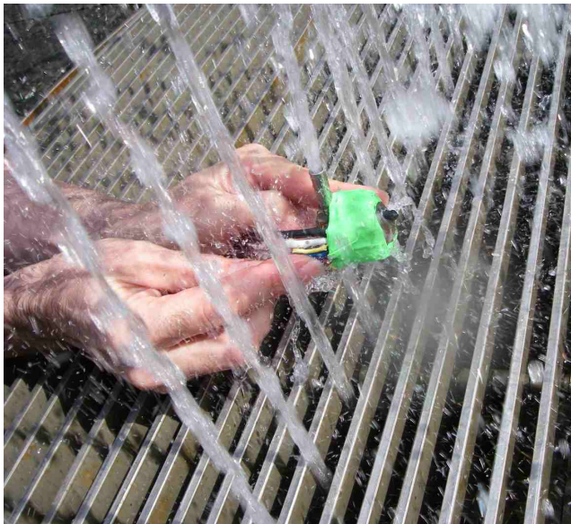
Figure 7: Hydrophone pickups held over water jets: In a computer-mediated world, each water jet is assigned to a different note on a musical scale. The computer vision system (wearable computer and EyeTap) is programmed so that the leftmost jet is the lowest note and the rightmost jet is the highest note. Sound from the hydrophone pickups is post-processed by filters in the computer that select out or emphasize harmonics in the sound that create the desired note, depending on input from the computer vision system. Because sound originates from the water, and is merely processed with computerized effects, this is not an electronic instrument (any more than is, for example, an electric guitar). The instrument affords a full range of musical expression and captures subtle changes in the way the hydrophones are held in the water jets.
