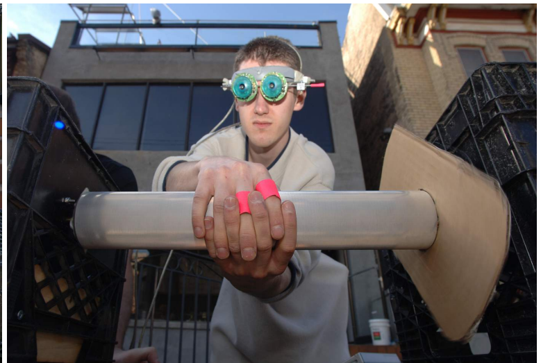
Figure 8: Polyphonic friction-idiophone having continuously variable pitch: A spinning aluminum cylinder with a specially textured surface produces sound picked up by a wireless contact microphone inside the cylinder. The sound is fed to one or more (depending on the number of fingers touching the cylinder) bandpass filters controlled by computer vision. The instrument can be used above or below the surface of the water.
