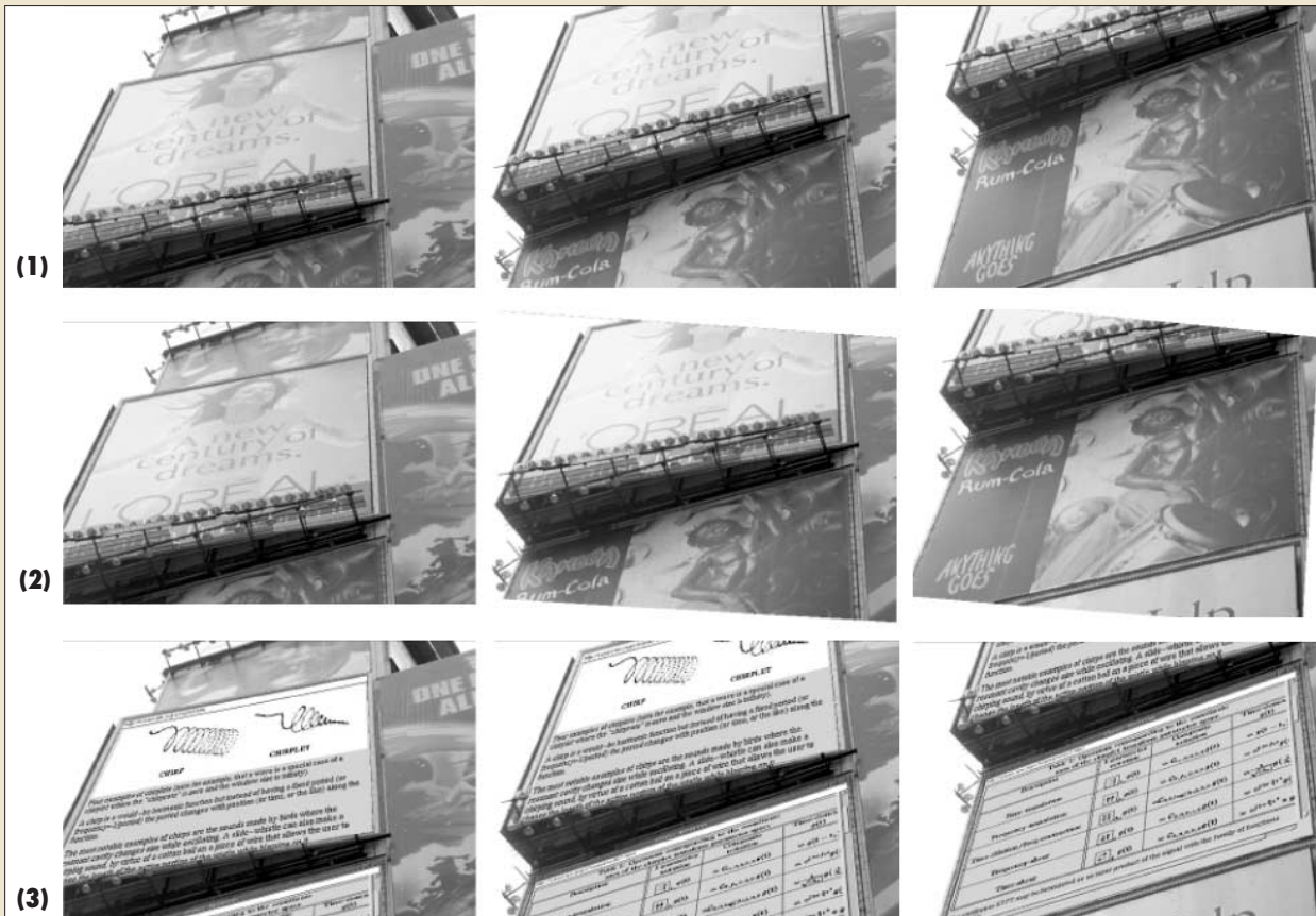
Figure A. Filtering out unwanted advertising messages (each row shows frames from a movie): (1) Advertising can be distracting and annoying. (2) A wearable computing device together with an EyeTap system (see the other sidebar) creates a modified perception of the advertising. (3) It then replaces the advertising with subject matter useful to the user.
