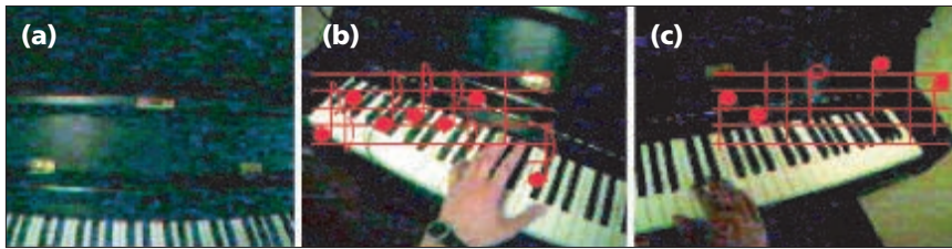
Figure 2. Views from the head-mounted display: (a) nothing overlaid when no hand is in view, (b) left-hand part displayed for the left hand, and (c) right-hand part displayed for the right hand.
