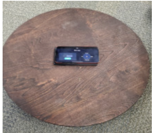
Fig. 1. Balancing board with IMU phone app used for game controls
