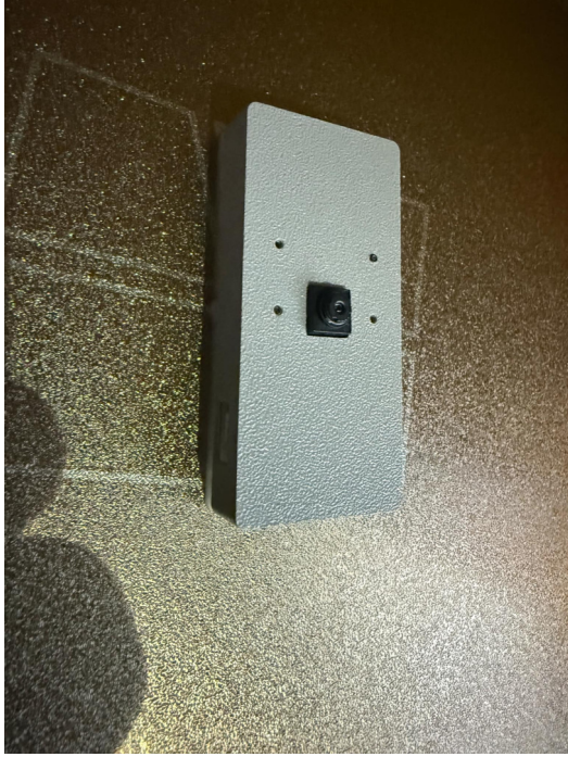
Fig. 1. Front view of the PETG enclosure showing Pi Camera mount and external fasteners.
