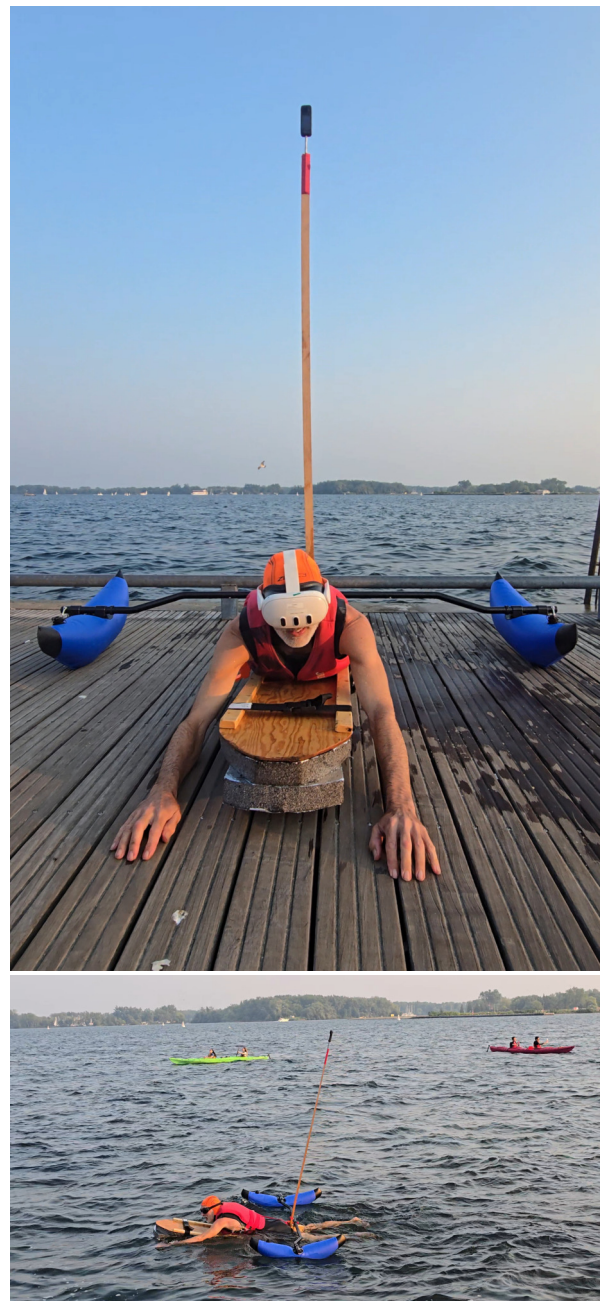
Fig. 21: Even a very narrow 12-inch (approx. 30cm) wide paddleboard can be made stable enough to support one or more tall masts, simply by adding outriggers. Here two outriggers convert the miniature paddleboard to a trimarin that can support up to 3 tall masts for visibility and safety.
