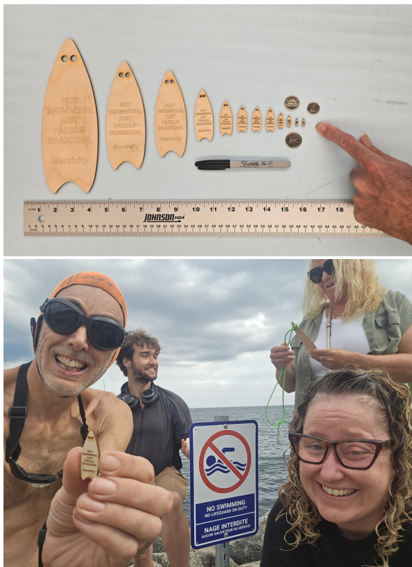
Fig. 18: Yoktoyachts™ lasercut/engraved in varying sizes to determine the smallest size with legible text.
