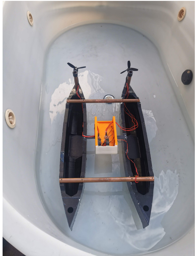
Fig. 6: Physical component of the autonomous watercraft made with CAD
