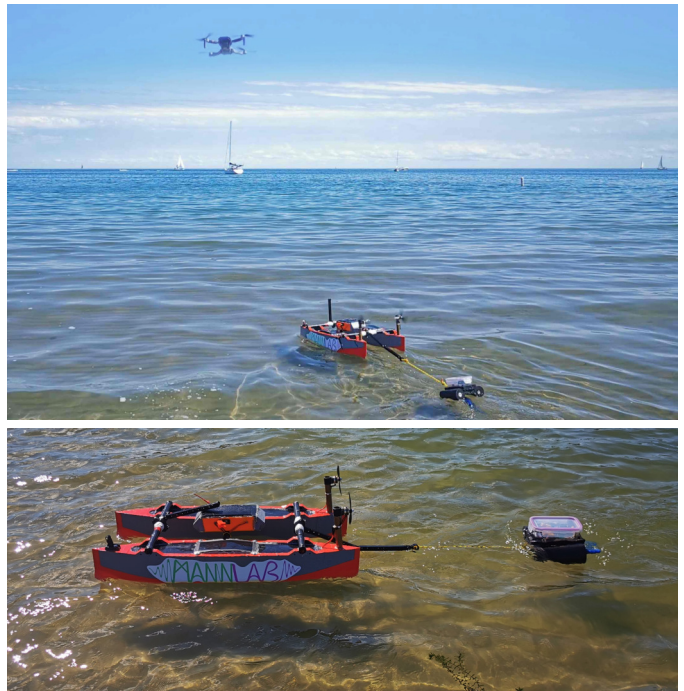
Fig. 7: Autonomous watercraft pulling the sensory and meta-sensory payload. An overhead drone tracks the autonomous watercraft's position within the body of water, based on the unique shape and color pattern of the watercraft.
