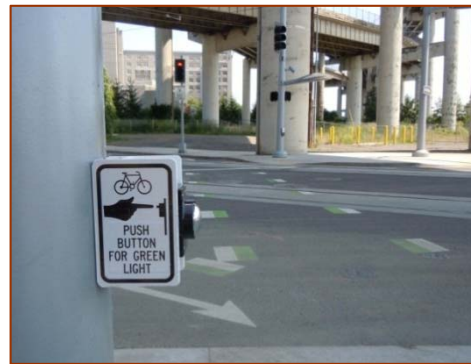
Figure 4.45 - Example of Cyclist Push Button
