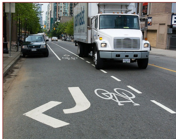
Figure 4.36 – Bicycle Lane Adjacent to Combined Right-Turn Lane
