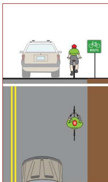
Figure 2.3 – Signed Bike Route (Rural Cross Section)
